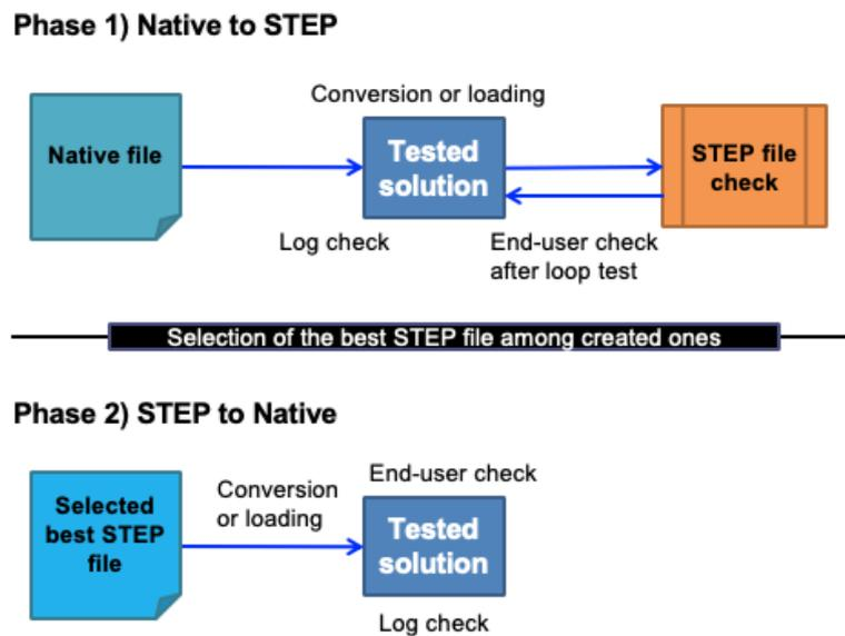
Figure 2 – Illustration of the CAD test procedure
